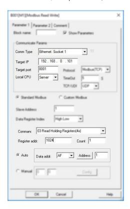
B004 is used to read the AI1 value from slave1, then save it into AF1 of master (slave1 IP 192.168.0.101, UDP port is 8001)
