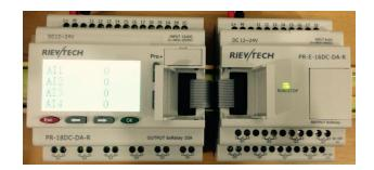
Figure 13 Connection the CPU with expansion
