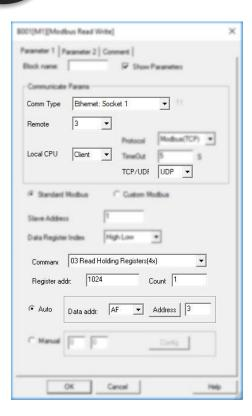
B006 is used to read AI1 value from slave3 and save the value into AF3 by UDP connection.
