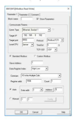
B002 is used to transfer the I1 status to the F1 of slave2 (slave2 IP 192.168.0.102, UDP port is 8002)
