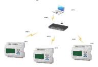
B.Directly communicate with other brand automatic components via TCP/IP connection based on MODBUS TCP protocol
